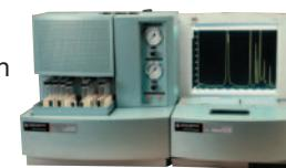
**Analect RefinIR™100t** oven accessory for data acquisition of heavy hydrocarbon samples at temperatures up to 100°C. Holds up to 12 40mL liquid samples and utilizes intrinsically safe sensors in concert with the Diamond 20 to perform analyses.
